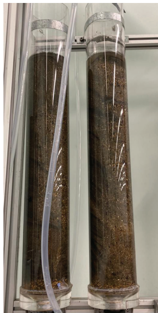
The two test column tubes were spiked with 250 mg each of PFOA and PFOS to mimic a PFAS source zone.
