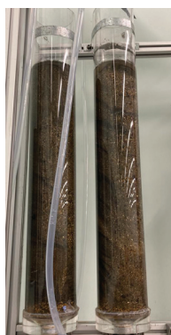
The two test column tubes were spiked with 250 mg each of PFOA and PFOS to mimic a PFAS source zone.
