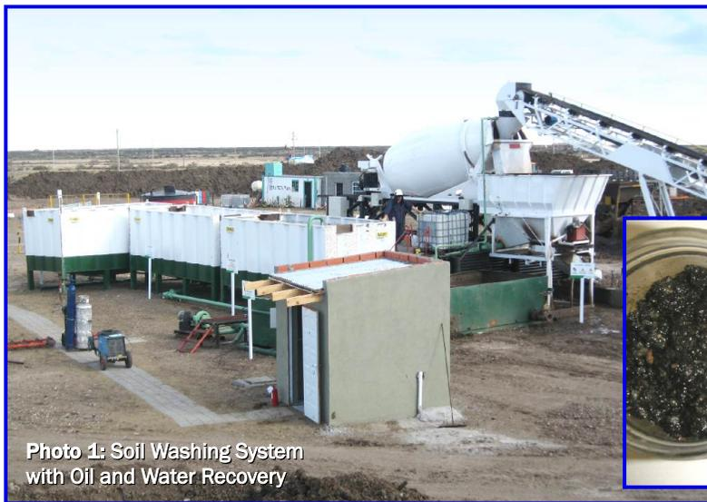
Photo 1: Soil Washing System with Oil and Water Recovery
