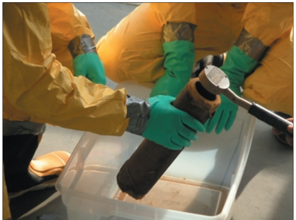
The concentrations that precipitate out in sludges and as scale on internal services of oil and gas production and processing equipment may vary in thickness from a few millimetres to more than an inch.
